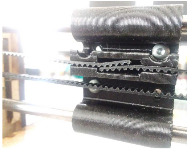
Figure 6.2: Mounting the timing belt to the pen holder assembly.
