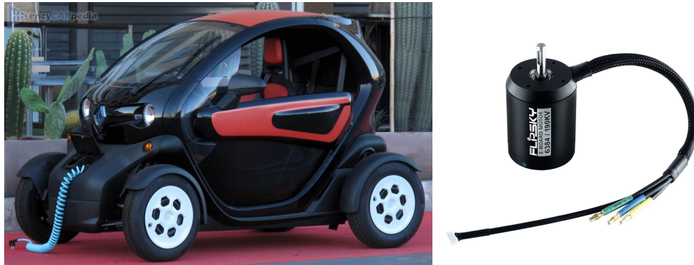
Figure 37.2: The Renault Twizy 45 (3730W) and a 6374 brushless motor from our parts catalog (3250W).
