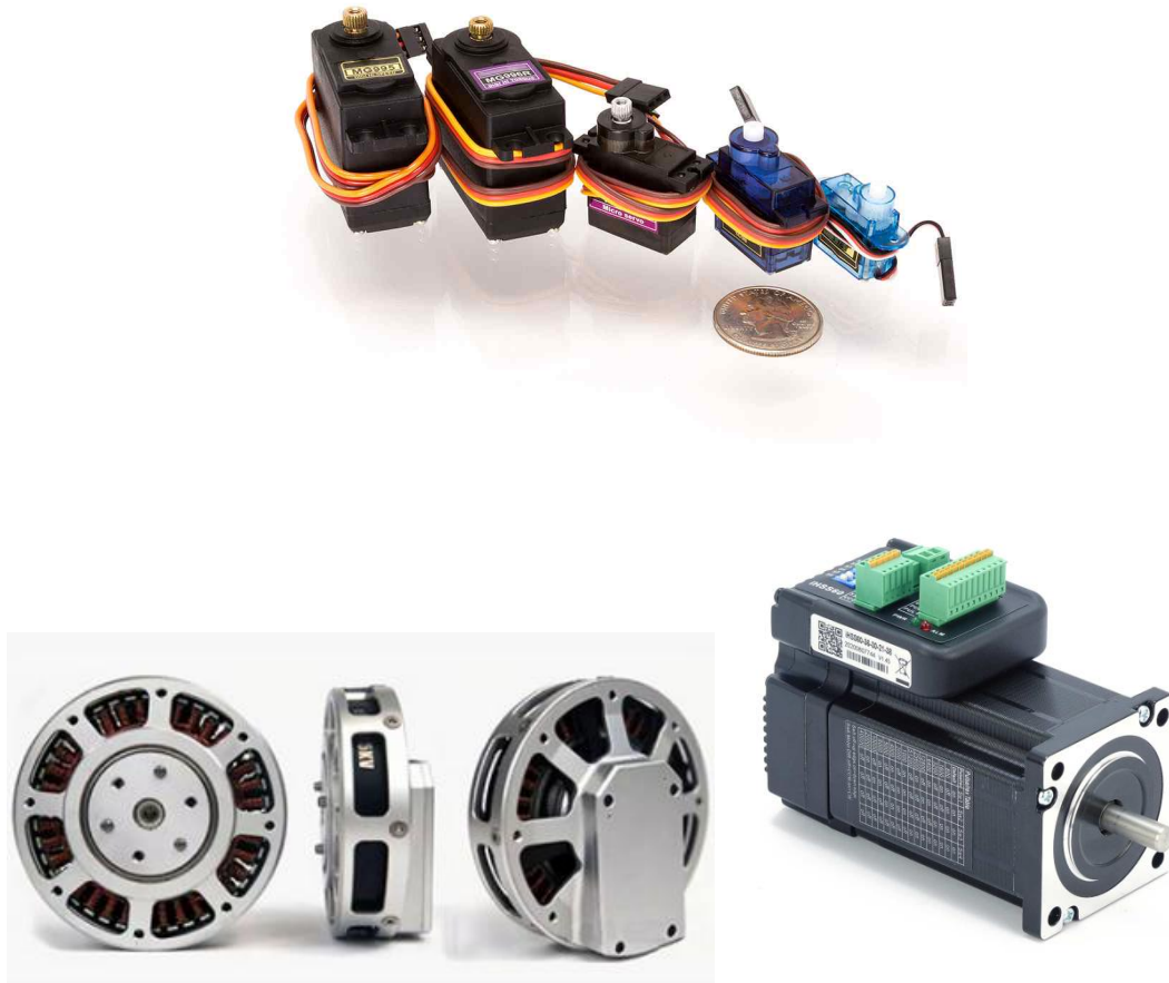
Figure 41.1: Brushed servos of different sizes in the popular box form factor (top), a brushless MIT robot dog servo (center), and closed-loop stepper (bottom).
