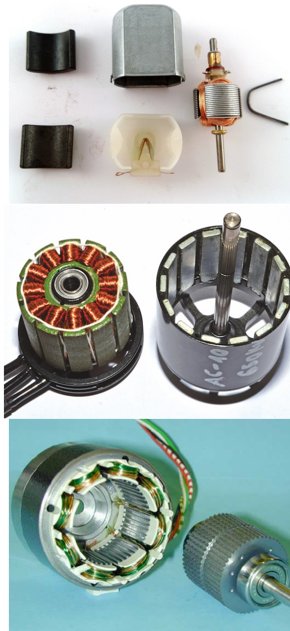
Figure 38.1: A brushed motor (top), a brushless motor with an external rotor (center), and a bipolar stepper motor (bottom), all opened up.
