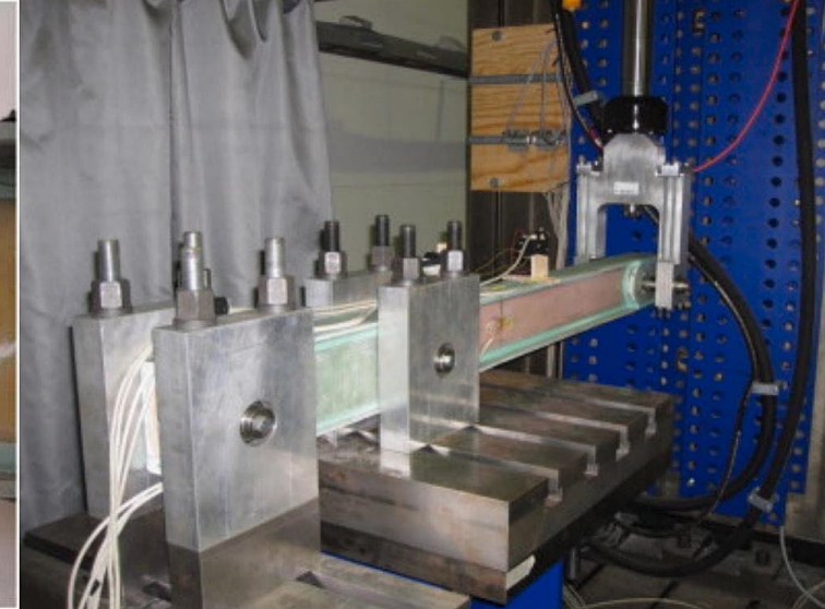
Adhesive bond failure between the spar beam and the flange in a wind turbine rotor blade [doi] (b) Henkel-Up Wind-Beam during cyclic test [doi] .
