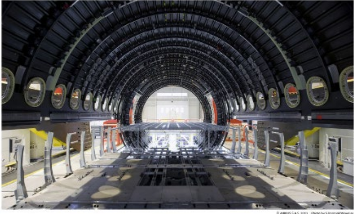
Aircraft fuselage longitudinal joint
