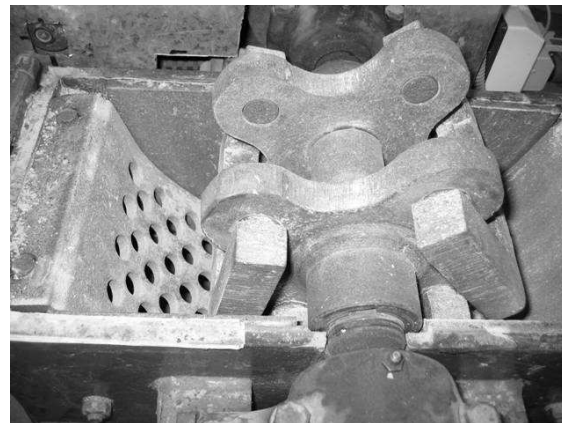
Fig. 2 Impactor: the material is crushed by the impact of steel pieces in rotation around the horizontal axis.
