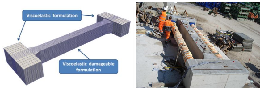
Fig. 7.22 Experimental specimen (right) and finite elements mesh (left)
