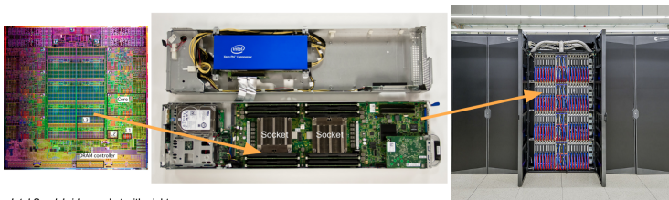
Intel Sandybridge socket with eight cores Stampede node with two sockets and a co-processor Server room
