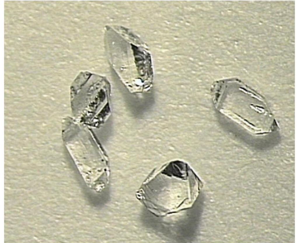
Fig. S1. Photomicrographs of [1(2,3)4] pentamantane crystals used for X-ray crystallography . Field of view, approx. 3.5 mm. Photograph, Marilyn Olmstead, U. C. Davis.
