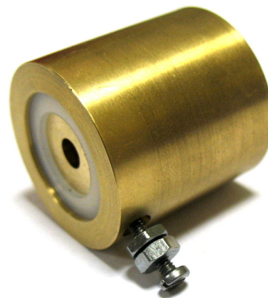
Faraday cup with an electron-suppressor plate in front
