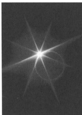
Fig. 3.16: Interesting non-collinear phase-matching effects in second-harmonic generation. (Picture taken by Rick Trebino.)
