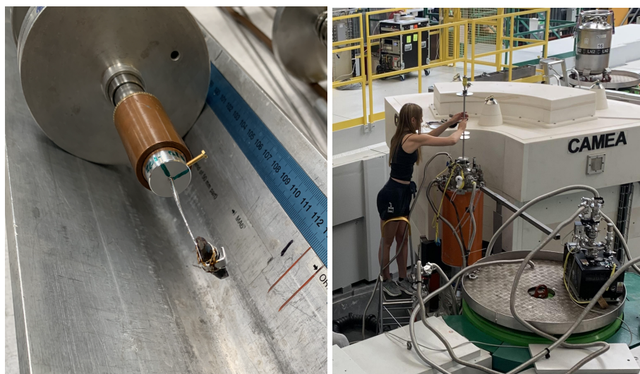
Fig. 4: (Left) Example picture of a sample mounted on the sample stick, (Right) The sample stick being inserted into the cryostat on the neutron instrument.
