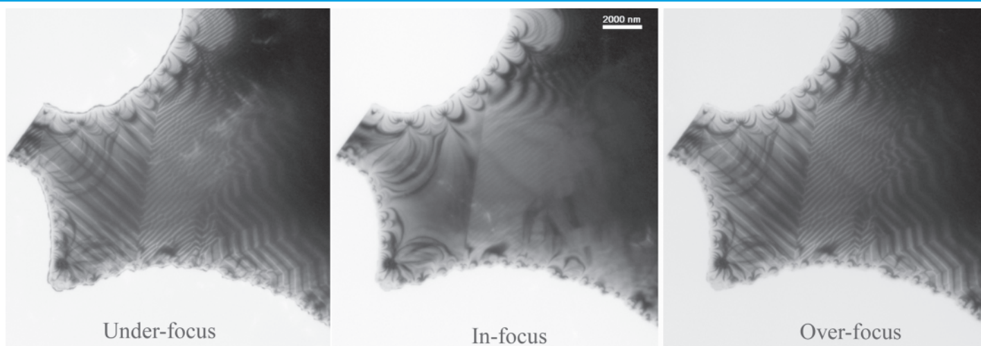
Figure 3. Lorenz microscope images of Perovskite-type manganese tri-oxide taken at under-focus, in-focus and over-focus conditions. The scale bar is 2 micron.
