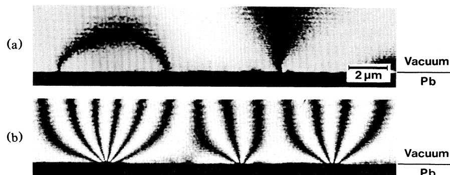
FIG. 1. Interference micrographs of magnetic fluxes penetrating superconducting Pb films (phase amplification, \times 2 ). Film thickness (a) 0.2 \mu\text{m} and (b) 1.0 \mu\text{m} .
