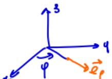
$$\vec{\omega} = \dot{\varphi} \vec{e}_z \quad \dot{\vec{e}}_\rho = \vec{\omega} \wedge \vec{e}_\rho = \dot{\varphi} \vec{e}_z \wedge \vec{e}_\rho = \dot{\varphi} \vec{e}_\varphi$$
