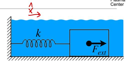
This represents the influence of an externally applied force with amplitude  $F_d$  and angular frequency  $\omega_d$
