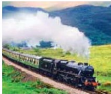
FIGURE 8-15 The burning of fuel (a chemical reaction) releases energy to boil water in this steam engine. The steam produced expands against a piston to do work in turning the wheels.
