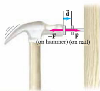
FIGURE 7-15 A moving hammer strikes a nail and comes to rest. The hammer exerts a force F on the nail; the nail exerts a force -F on the hammer (Newton's third law). The work done on the nail by the hammer is positive ( W_n = Fd > 0 ). The work done on the hammer by the nail is negative ( W_h = -Fd ).
