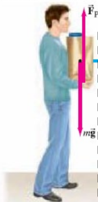
FIGURE 7-2 The person does no work on the bag of groceries since \vec{F}_P is perpendicular to the displacement \vec{d} .
