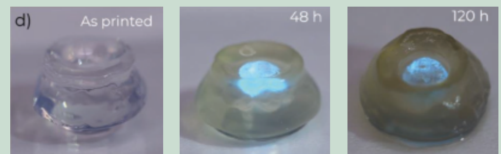
Figure 5: Printed structure showing the evolution of darkening of the outer shell and bioluminescence of the filling when in contact with IPTG
