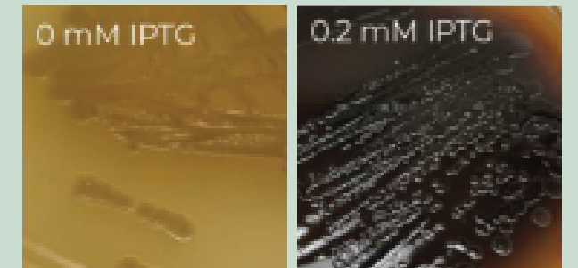
Figure 4: Genetically modified E.coli containing hydrogel with (right) or without (left) being in contact with IPTG
