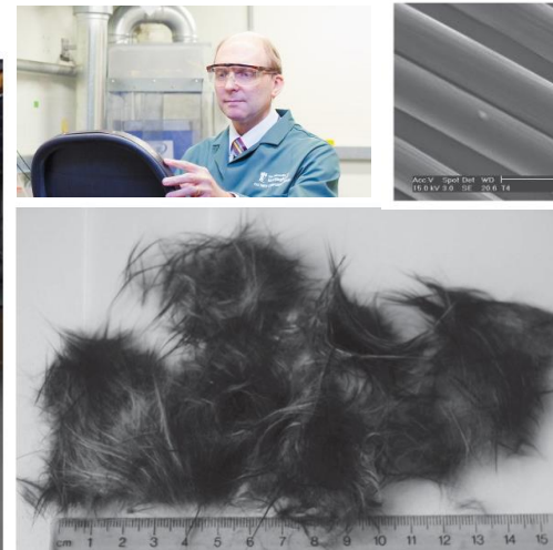
Figure 4. Recycled carbon fiber in a fluffy form.
