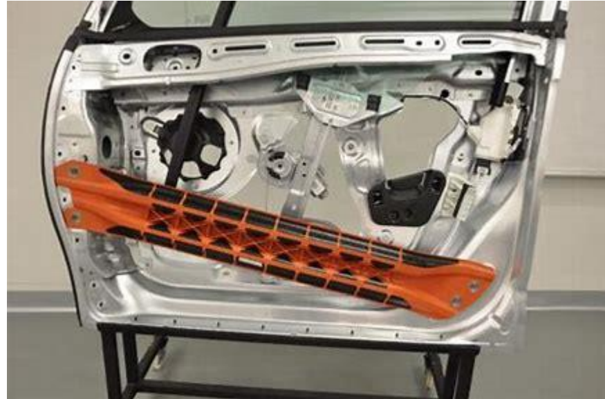
PSA Side Intrusion Beam development with overmolded DuPont Vizilon™ TPC sheet, JEC Paris, March 2013
