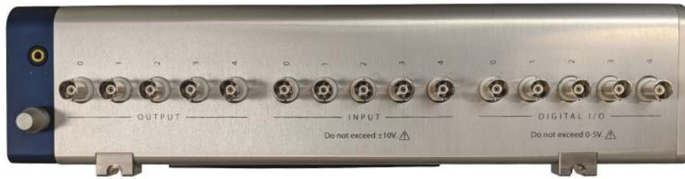
Figure 4.2.: Side view of Backpack Controller showing BNC connections.
