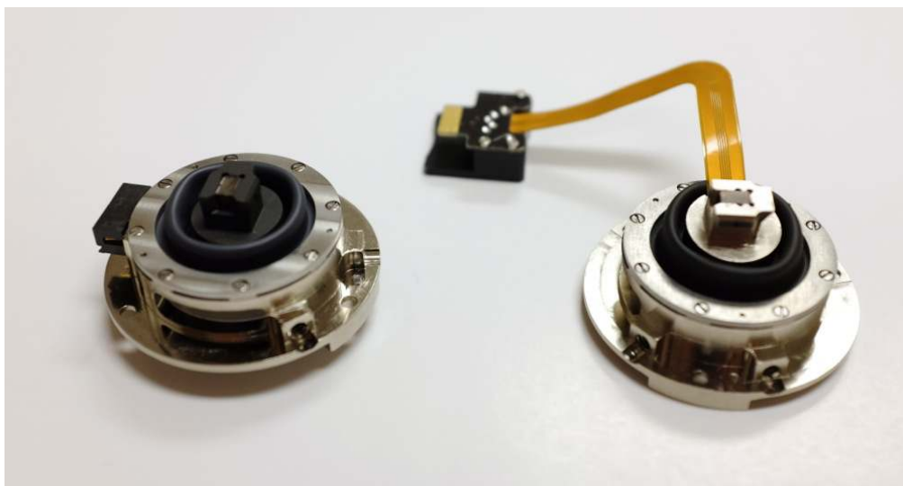
Figure 19.7.: Ambient stage / fluid cell body combination on the left. Heater stage / Gas cell body combination on the right.
