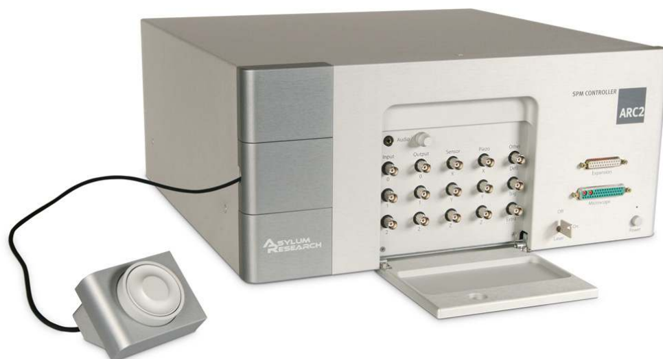
Figure 3.1.: The ARC2 Controller with Hamster extended and BNC connector hatch open.
