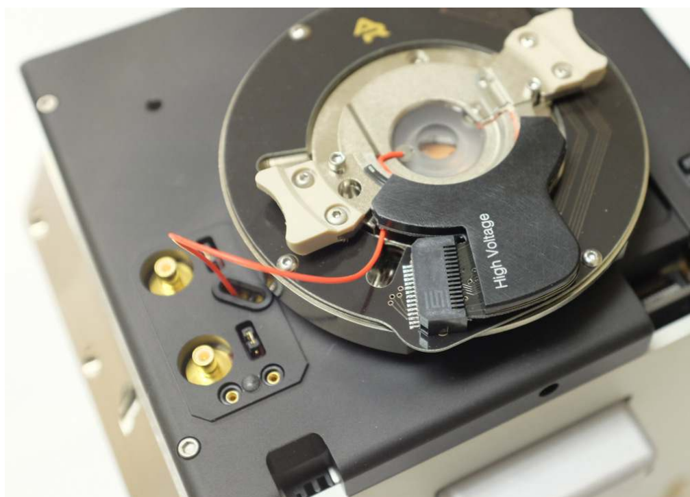
Figure 24.2.: High Voltage Scanner with High Voltage cantilever holder and its fly wire connected to the high voltage contact.
