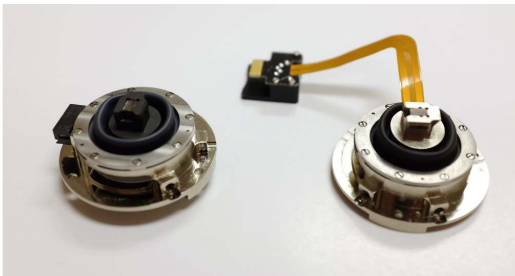
Figure 19.6.: Ambient stage / fluid cell body combination on the left. Heater stage / gas cell body combination on the right.
