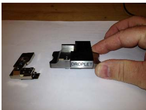
(a) Droplet Cantilever Holder Changing Station XXX.XXX. Notice the markings.
