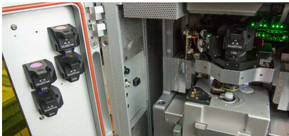
Figure 34.4.: Spare Filter Cube docked on the Cypher door.
