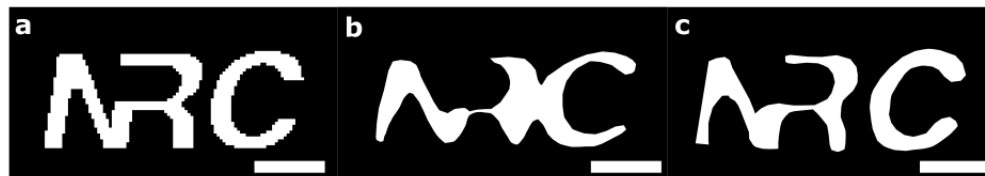
Fig. 9. Jaccard similarity index determination for the custom part in Fig. 7. Binary images of a cross-sectional slice through (a) the target model, (b) the part fabricated using a 16 mm aperture with the Radon method, and (c) same as in (b) but with 3DRT. All scale bars are 1 mm.
