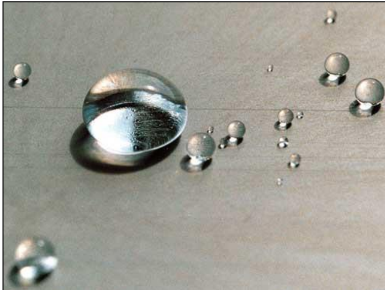
Stainless steel with an abrasion resistant fluorinated hybrid coating
