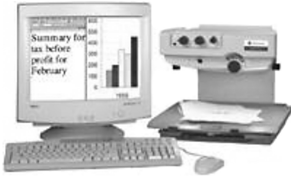
Figure 2. Closed-circuit television with computer based text-to-speech output, a talking computer.
