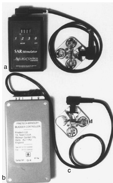
Figure 25. External equipment. (a) New control box. (b) Original control box. (c) Transmitter lead. (d) Transmitter block.
