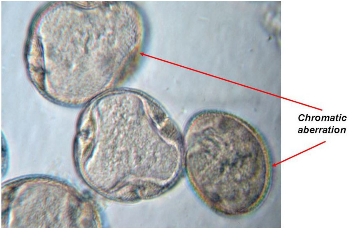
Tilia (European Lime) pollen X60 planapochromat objective Canon G9 super widefield eyepiece, showing chromatic aberration (colour fringing)
