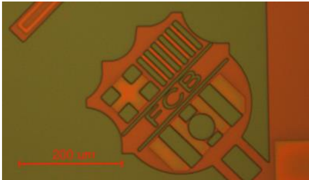
Figure 8 Example of a fancy design, the FC Barcelona crest, realized during a past practical, right before the SiO 2 etching step. In that case the Cr tracks are open and the cantilever can't be actuated. Green: SiO 2 unprotected; orange: SiO 2 covered by PR; orange with shades: SiO 2 covered by Cr and PR.
