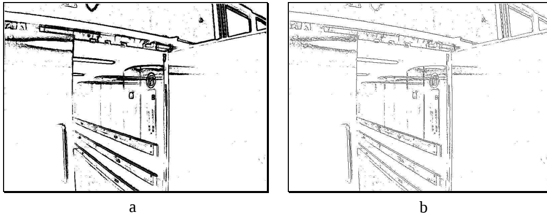
Fig 4.43 (a) Edge image of the Figure 1.2(b); (b) Non-maxima suppression of (a)
