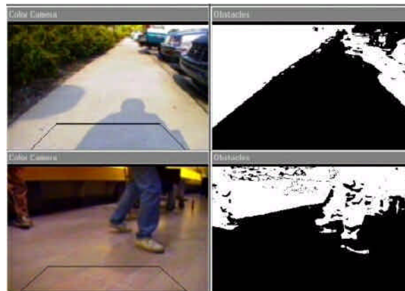
Fig 4.46 Examples of adaptive floor plane extraction. The trapezoidal polygon identifies the floor sample region.
