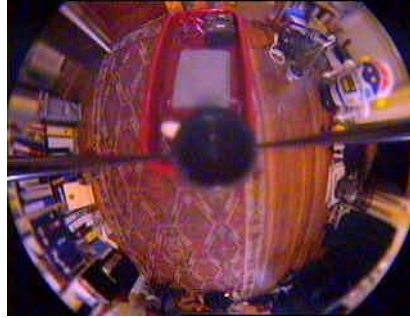
Fig 4.48 An image acquired by the OmniCam catadioptric camera system.
