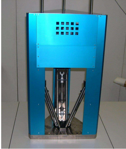
a) Vertical linear delta with 3 columns
