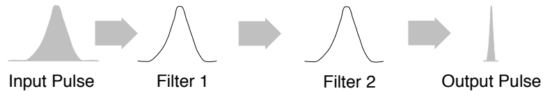
Figure 335. Effect of Multiple Filters on Signal Pulse
