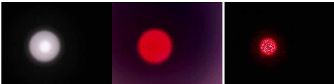
Figure 26: Example images of the light output of the multimode fibre for three different sources (left) Halogen lamp, (middle) LED and (right) laser. (Not at the same distance!) Please take care that the images are well centred.
