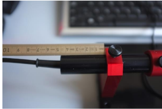
Figure 23. Position of the LED source to achieve a high NA focalisation. The distance from the fibre to the lens is approximately 20 mm. The lens diameter is 9 mm.
