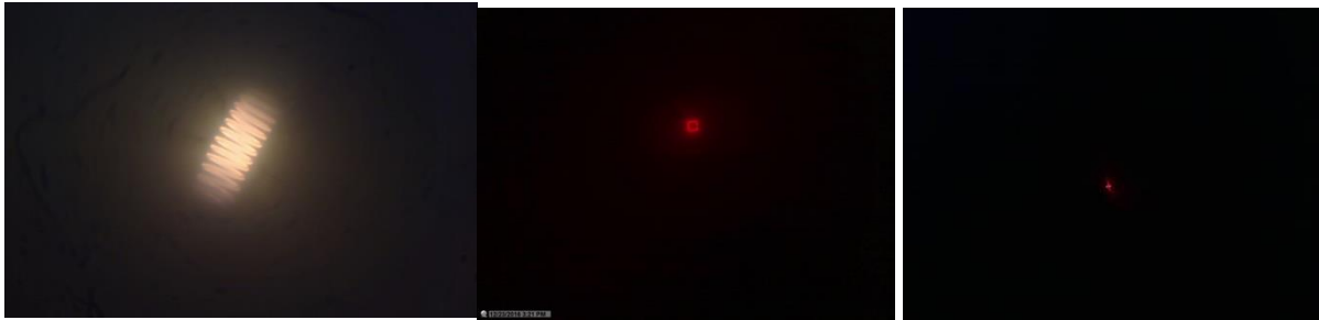
Figure 11. Minimum focus spot obtained using different light sources. The laser can be focused on a very small spot. The LED has a larger size and the chip is visible. The halogen lamp is biggest. The field of view is 4.536mm x 3.416mm.
