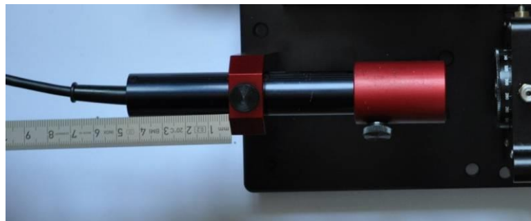
Figure 28. Position of the LED source to achieve a high NA.
