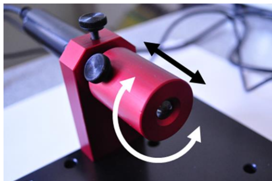
Figure 14. Focalization (black arrow) and intensity adjustment with the lens cap.
