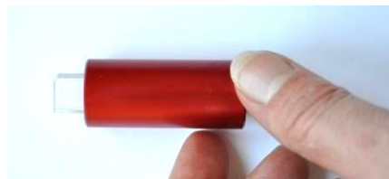
Figure 13 The beam splitter is a 10 mm cube mounted on a cylinder.
