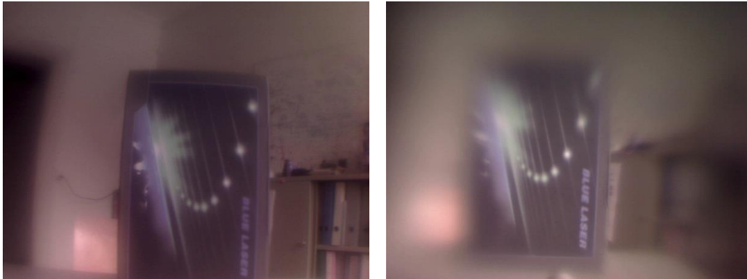
Figure 1. Images taken with a planoconvex lens when the curved surface is oriented towards the detector (left) and towards the object (right). One sees a large difference between both images.
