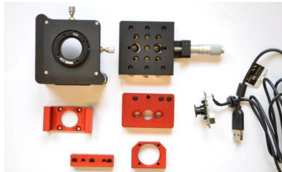
Figure 12. Parts used in this experiment. The 6-axis stage with x-y positioning, rotation and angular adjustment. The linear stage to set the distance precisely and parts for adjustment.
