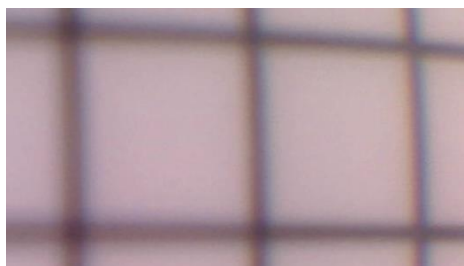
Figure 26. Example images to demonstrate chromatic aberrations. The defocused image shows color effects at its outmost areas.
