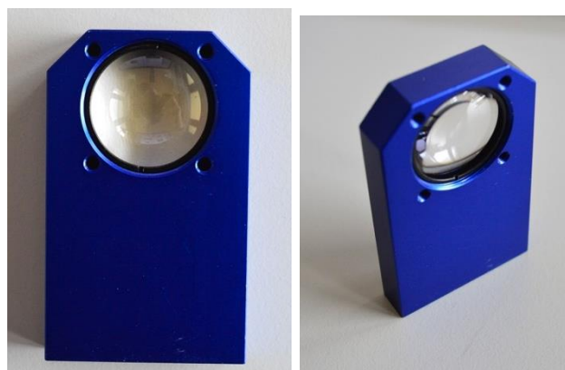
Figure 24. The second biconvex lens ( f=25.4 mm) needed for the double lens arrangement in its holder.
