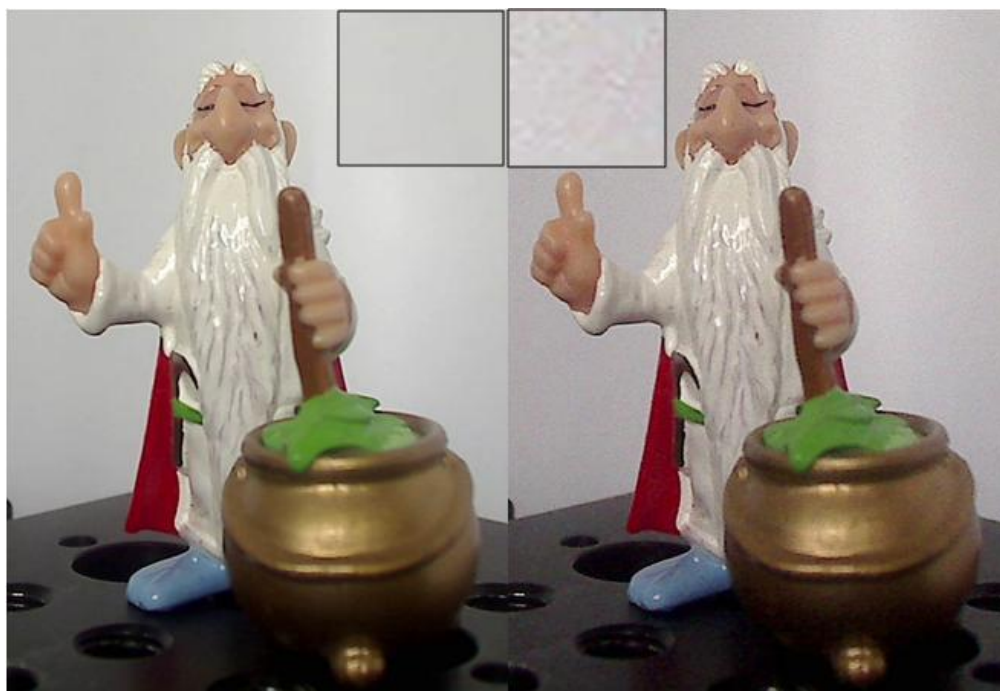
Figure 1 The same image taken at different amplification values: Left: low gain and right high gain. The inset shows the effect of electronic noise on the image quality.
