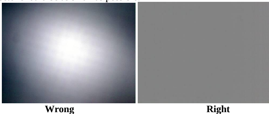
Figure 11. Two cases of intensity variation over the detector surface. The left is badly adjusted, while the right shows a high uniformity.
