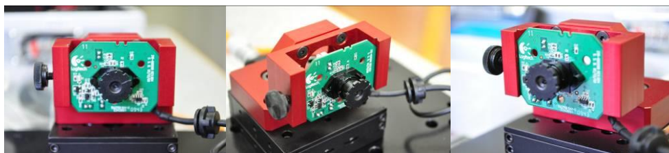
Figure 9: Camera PCB in the mount ready for shooting.
