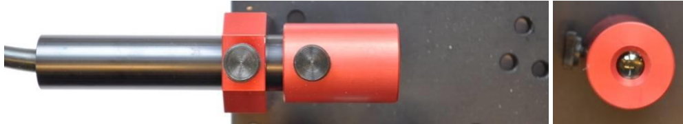
Figure 20: Source mounted with the lens cap (on the right) to achieve focusing and collimation
