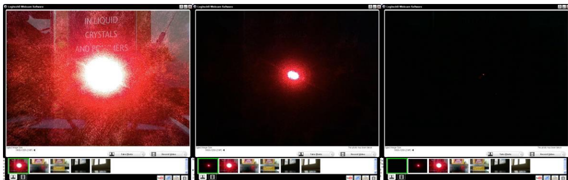
Figure 23: Left: Overexposed image by using automated exposure. Middle: Image with lowest gain and shortest exposure time. Right: Image of the focal spot without saturation at highest attenuation.
