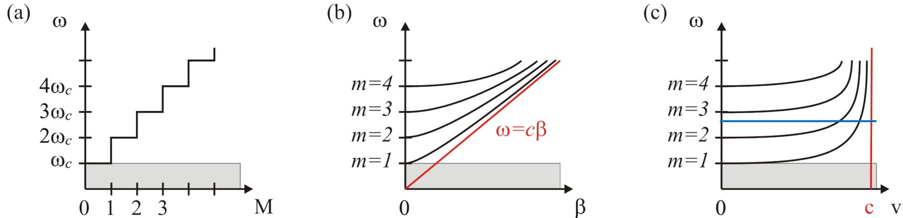
$$\beta_m^2 = \frac{\omega^2}{c^2} - \frac{m^2 \pi^2}{d^2} \quad \beta_m = \frac{\omega}{c} \sqrt{1 - m^2 \frac{\omega_c^2}{\omega^2}}$$
