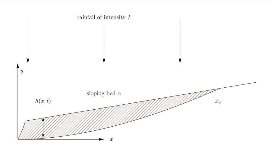
7. Let us consider the kinematic wave approximation for a water flow induced by rainfall of intensity I over a sloping bed (starting from  $x_0$ )
