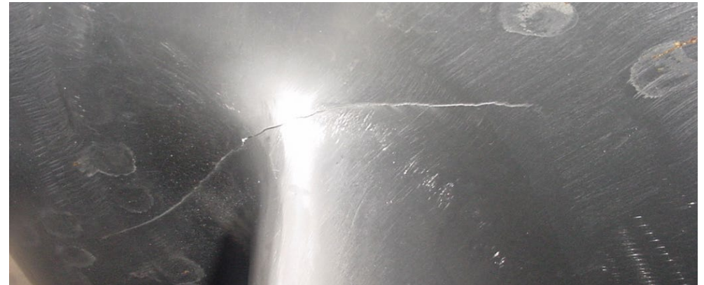
Severe erosion in pump propellers
