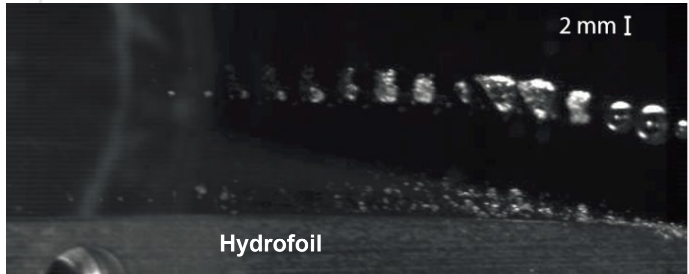
Figure 3.18: Case 3 : Superposition of the high speed images of the collapse of a bubble generated at (-5, +9) . The bubble has a microjet not towards the solid surface. Interframe time: 180 \mu\text{s} , maximum diameter: 5 mm, bubble lifetime: 440 \mu\text{s} .
