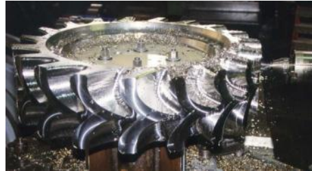
Pre milling of coupling and NC milling of buckets roots
