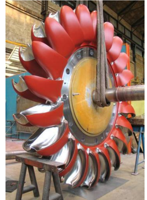
Grinding and polishing of the buckets
