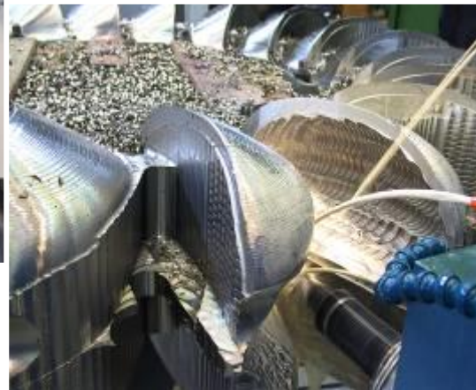
CNC machining of the buckets and runner hub
