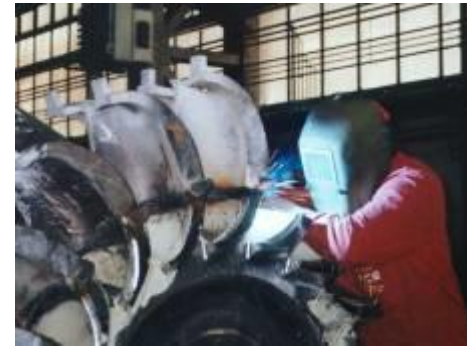
Hiweld™ welding of middle parts
