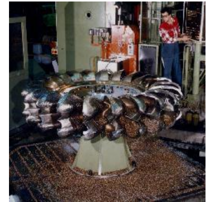
NC milling and final grinding
