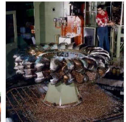
NC milling of bucket profile and final grinding
