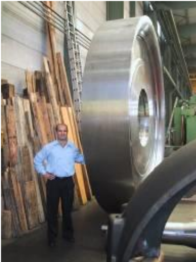
Forged disk with pre milling
