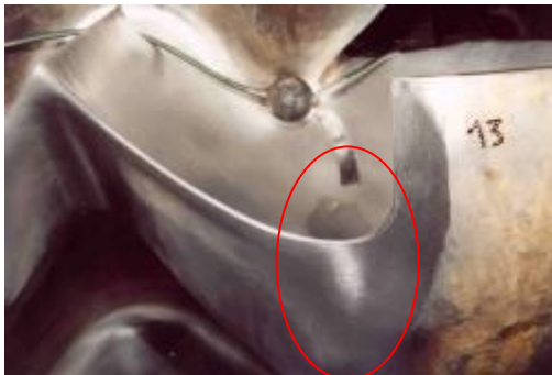
Damages on buckets
