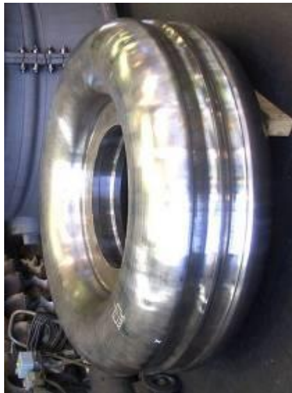
Forged disc pre machined and checked by UT
