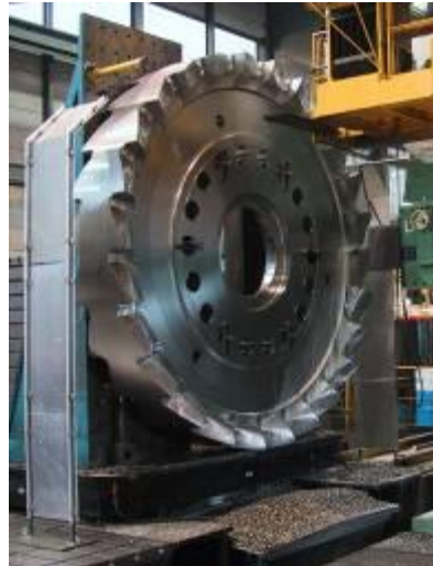
Pre milling of coupling and NC milling of buckets roots
