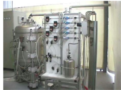
Figure 1: Schematic and realistic views of an industrial continuous stirred tank reactor.
