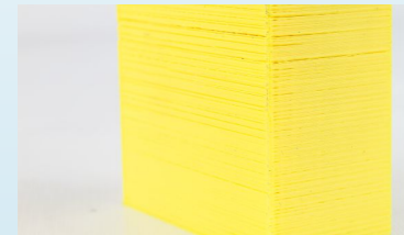
Layer Separation - matterhackers.com
