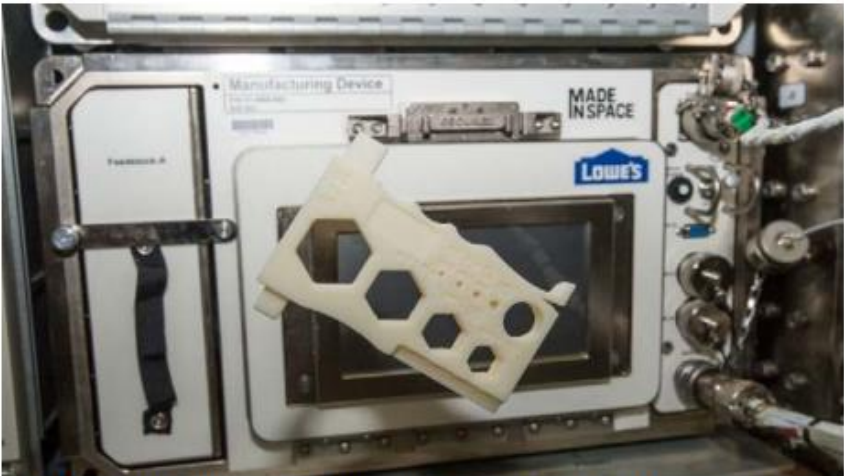
AMF on ISS with printed multi-purpose tool floating in front (photos courtesy of MIS)
