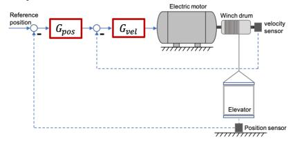
A control engineer has identified the following transfer functions in the system:  $\frac{Y_{el}(s)}{\Omega(s)} = \frac{0.5}{s}$  and
