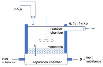
For the parameter values: reactor volume  $V = 3 m^3$ , feed flow rate  $q = 0.25 m^3/min$ , mass transfer coefficient  $k_m = 1.5 m/min$ , and input feed concentration  $C_{Ai} = 10 \ kmol/m^3$ :
