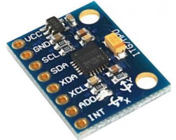
MPU6050 Accelerometer + Gyroscope
