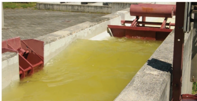
Fig. 1. (Color) Experimental AMIL gate exhibiting oscillating behavior and creating waves
