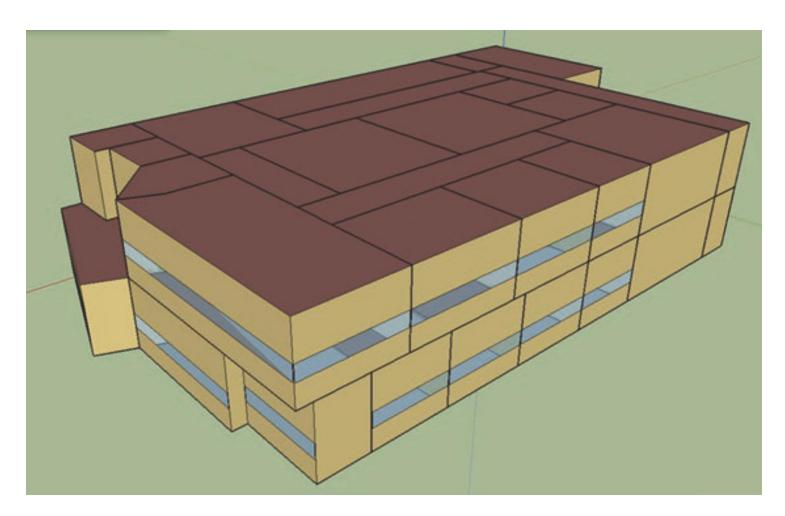
Simplification of detailed building geometry
