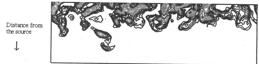
Fig. 9.1. Contours of the kinetic energy on one plane in the flow created by an oscillating grid in a large body of quiescent fluid; from Briggs et al. (1995)
