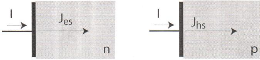
Figure 5.5: In the absence of net generation or recombination at an ohmic contact, terminal current is entirely supported by the majority carriers in the semiconductor (n-type on left, p-type on right).
