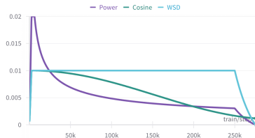
Figure: Example Warm-up+Runtime+Cool-down schedules vs. cosine annealing schedule. Credit: [48].
