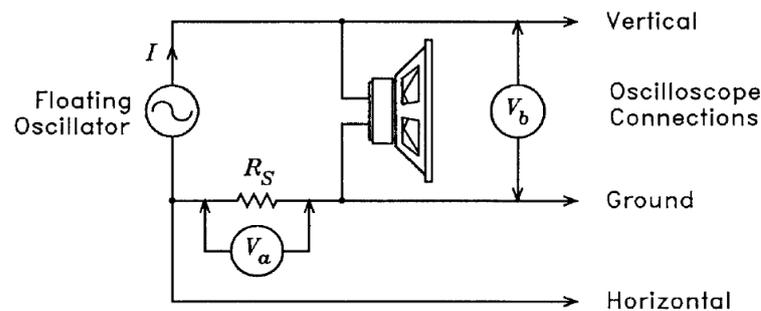
The input impedance is deduced from the known measurement resistance  $R_s = 1\Omega$ , as  $\hat{Z}_{hp} = R_s \frac{V_b}{V_a}$  and gives the following result :
