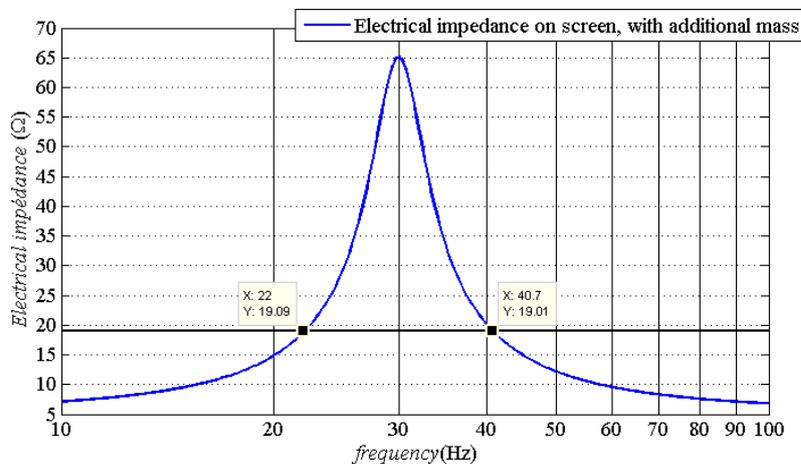
The measurement gives the two new frequencies  $f'_1 = 22Hz$  and  $f'_2 = 40.7Hz$ .
