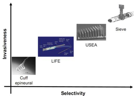
Fig. 1. Types of peripheral nerve interfaces [3]
