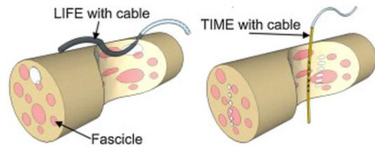
Fig. 3. Intrafascicular electrodes LIFE and TIME [6]
